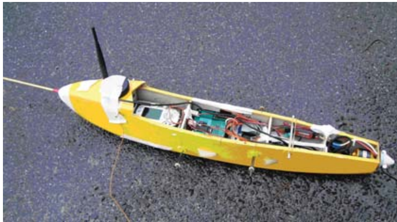
Fig. 7. Positions of equipment items in the miniBSP airframe
